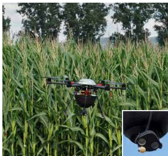
Application of Trichogramma capsules with a GPS-controlled multi-copter.
